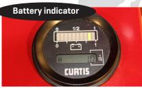
Battery indicator and hour indicator for hours remaining before next service.
